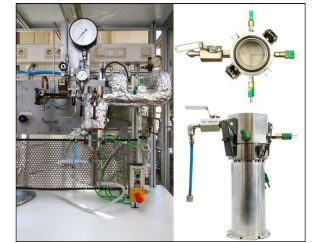
Figure 4. Lab-scale steam pressure filtration rig
