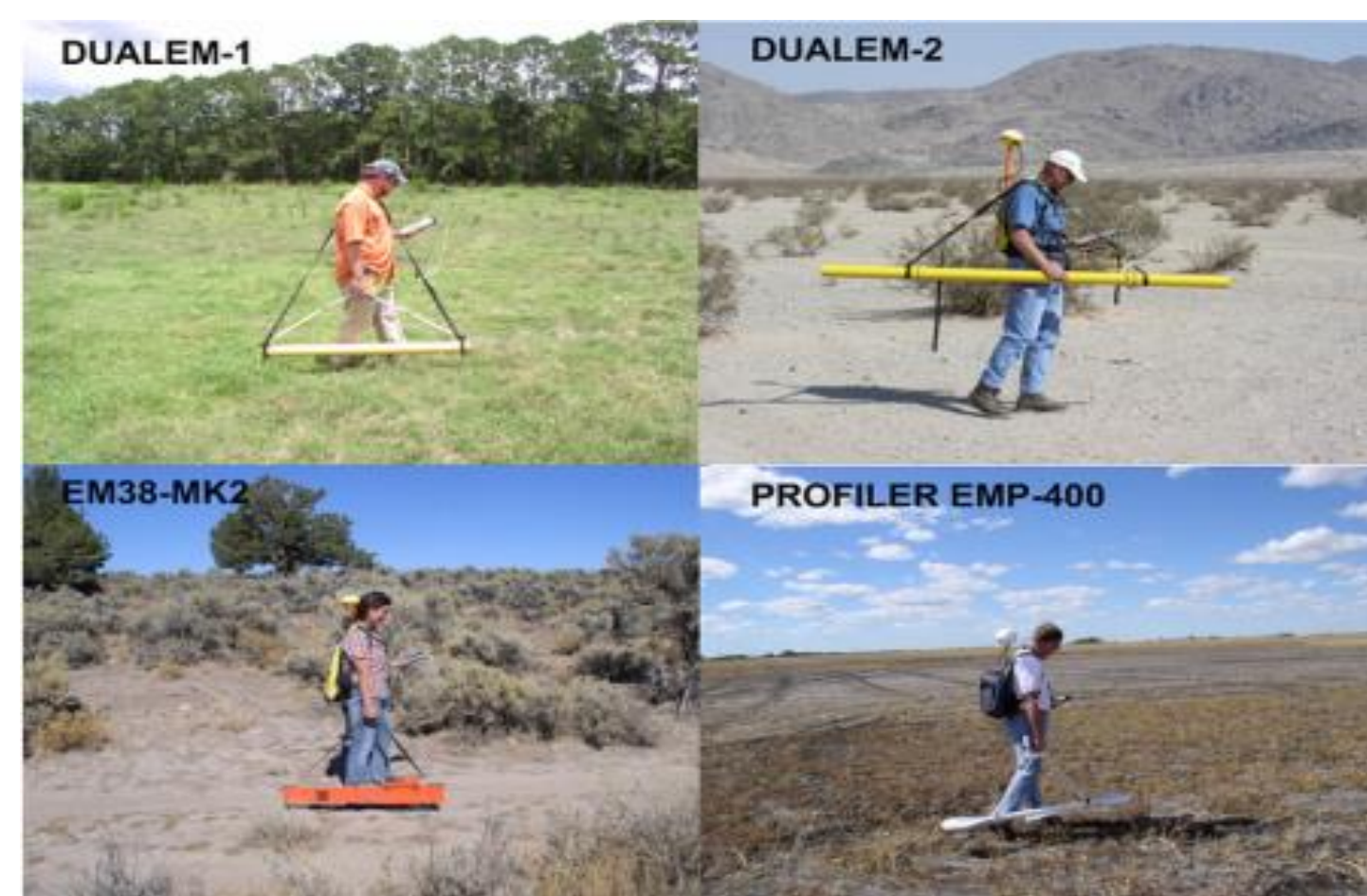
Figure 2: EMI equipments are easy to move and compact (Doolittle and Brevik, 2014)
