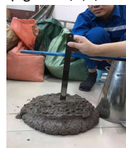
Fig 3. Material slump testing
